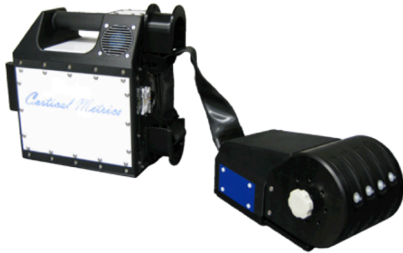
Figure 1. CM4 vibrotactile stimulator.
